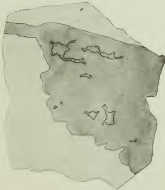
FIG. 9—Specimen of siliceous ore from Penobscot mine, Black Hills, South Dakota. Shows wavy lines of demarcation between ore (dark) and limestone (light). About half natural size.
